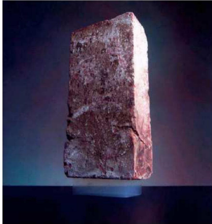
Fig 1. A 2.5 kg brick is supported on top of a piece of aerogel weighing only 2.38 g. (NASA)
